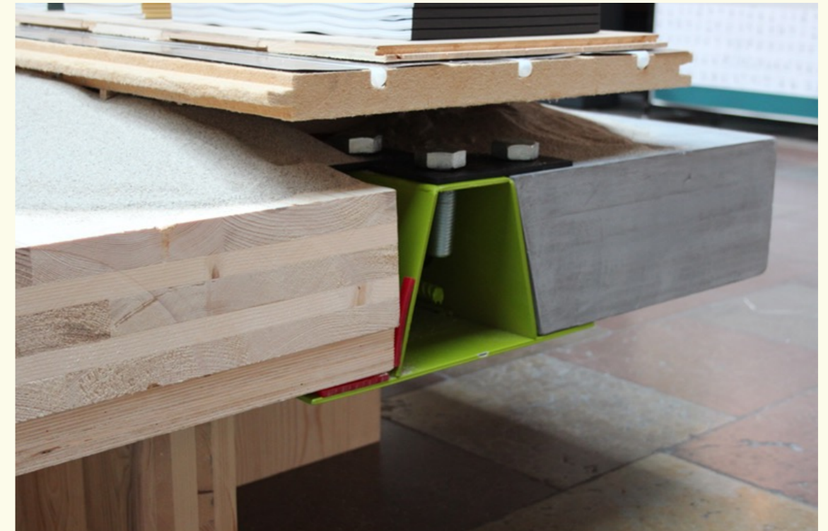
Figure 3.2: 1:1 Model of DfD floor slab
